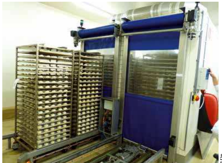
++ Pairs of rack trolleys are driven automatically into the proofing room, where they remain for 60 minutes
