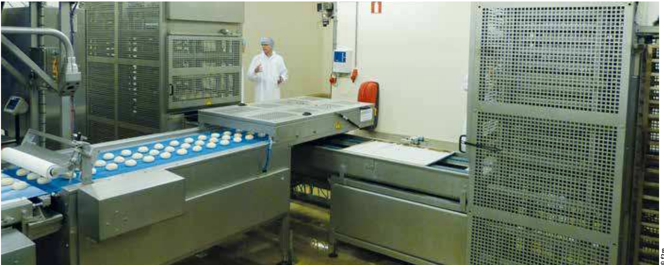
++ The filled dough pieces are deposited onto trays. Input and removal take place automatically. The entire project was designed by the Kortlever company
